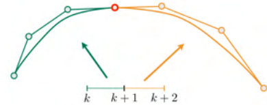
Figure 8.2. Enforcing continuity constraints on Bézier curves: C^0 , C^1 , and C^2 cases, respectively
