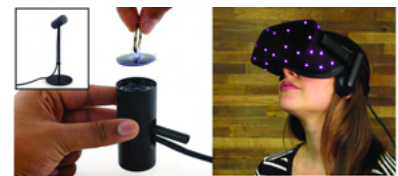
Figure 24.3. Oculus rift IR LED tracking hardware
